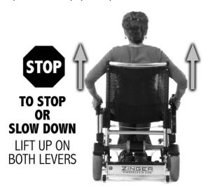
**NOTE:** Remember that the brakes will always apply when both levers are pulled back. If you have any confusion, just pull up on BOTH levers to brake!
