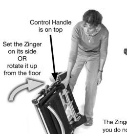
To carry, grab the base frame tube with your right hand where the Keep Tires Inflated label is. Keep the underside of the Zinger facing away from you as shown on the right. It will balance from one hand.
