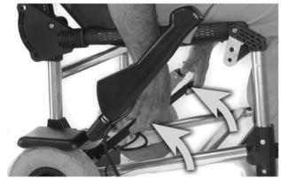
**HINT:** Most users find it easiest to reach inside the Control Levers to access the Parking Brake Levers, as shown in this photo.
