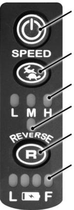
Power Button (Press and wait three seconds. Indicators below will light when ON.)
